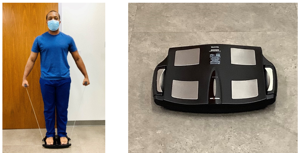
Figure 3. Home-based bioimpedance device; photo courtesy of Clifton J. Holmes, PhD.
