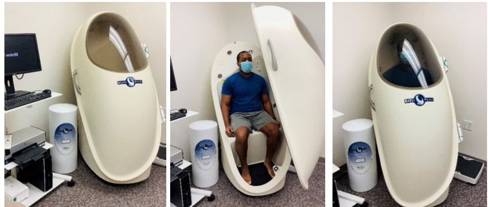
Figure 4. Air displacement plethysmography via BOD POD; photo courtesy of Clifton J. Holmes, PhD, in conjunction with the Pediatric Clinical Research Unit at the Washington University School of Medicine in St. Louis.
